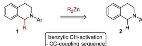
Figure 1. Proposed sp 3 -CH-activation cross-coupling strategy of THIQs with organometallic reagents.
